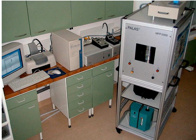
MFP2000 system for testing of filter material (PALAS GmbH)
