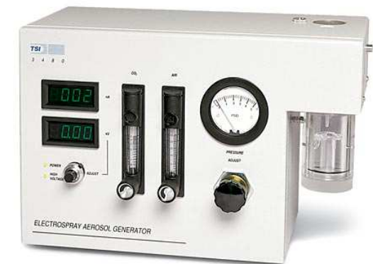
Electrospray monodisperse aerosol generator (TSI Inc.) 2-500 nm
