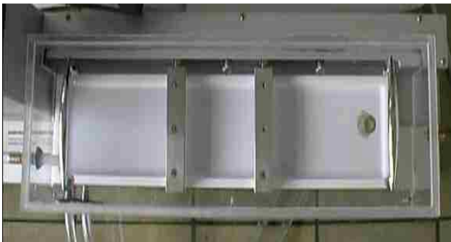
Langmuir-Wilhelmy balance Minitrough (KSV, Finland)
