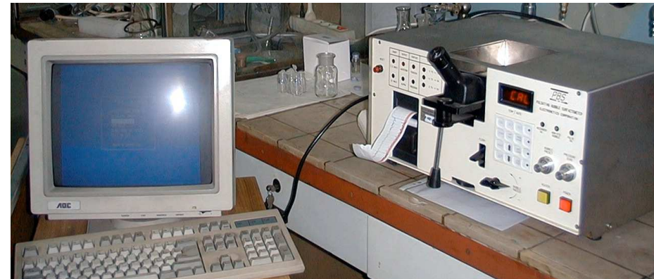
Pulsating Bubble Surfactometer (Electronetics Corp, USA)
