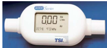
Digital flowmeters (TSI Inc., USA)
