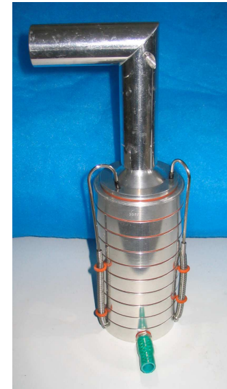
Andersen-type cascade impactor (Copley Sci., UK)
