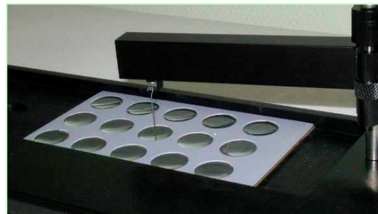
Needle microtensiometer (Kibron, Finland)
