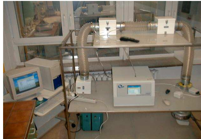
wide-range aerosol spectrometer XPS, 10-500 nm (MSP Inc., USA)
