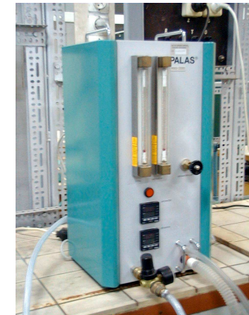
oil mist generator (PALAS GmbH)
