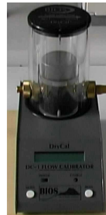
Flow calibrator (BIOS Inc., USA)
