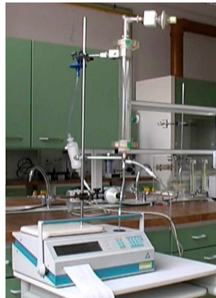
laser particle counter (A3 GmbH)
