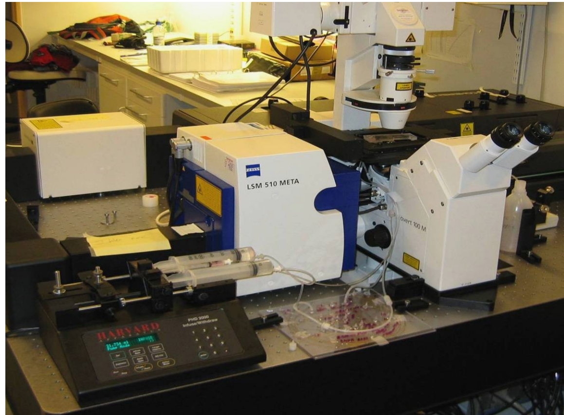
Laboratory setup (Confocal Laser Scanning Microscopy)
