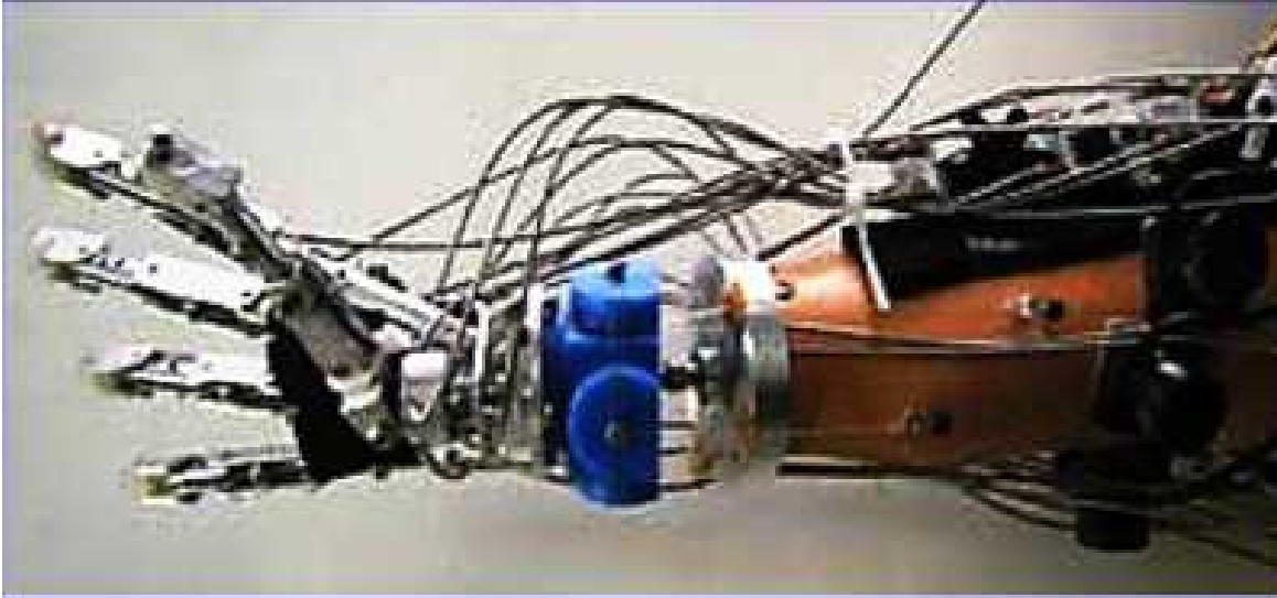
Prosthetic hand powered by SMA actuators, after Fig. 16. in Jani (2014)
