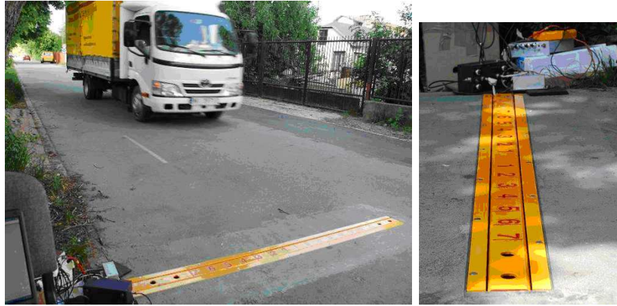
Figure 2.23: Second version of the beam-shape WIM device mounted on public road
