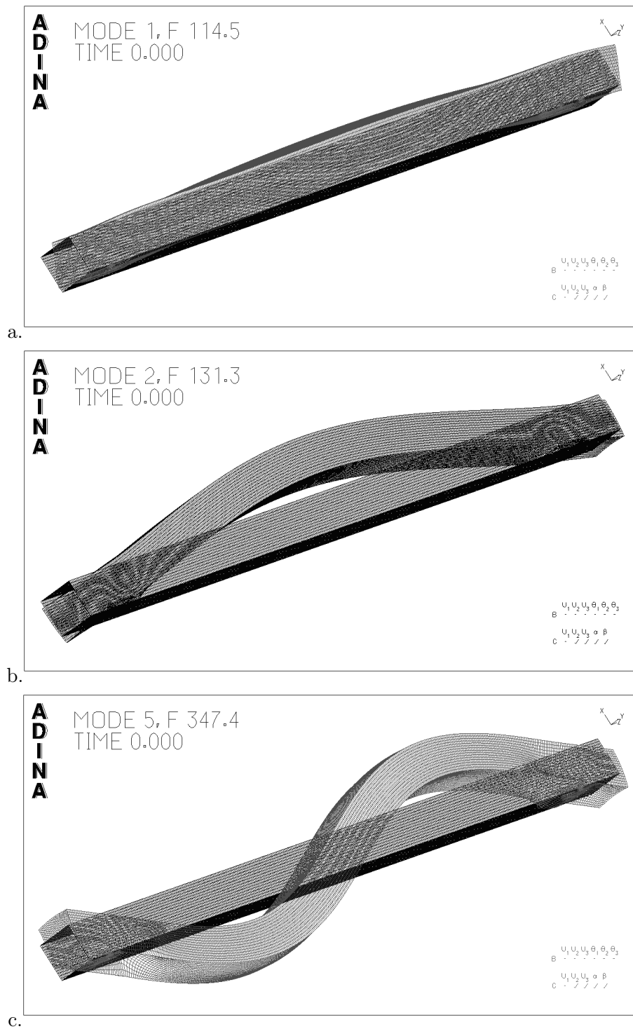
Figure E.1: Modal shapes of the beam-shape structure: a. mode I, b. mode II, c. mode V
