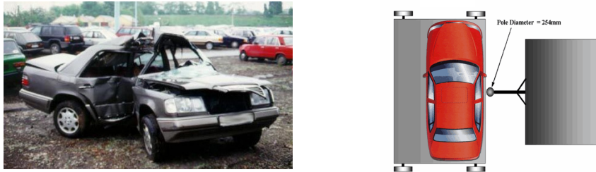
Fig.5.1.14: Lateral impact thin-walled door of the passenger car: a) deformation of the car after lateral impact with high velocity, b) scenario of NCAP 'Pole side impact' test
