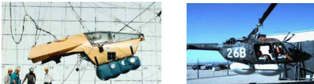
Fig.6.2.1. System of external airbags: a) F-111 crew escape module equipped with an external airbag [298], b) emergency airbags attached to helicopter undercarriage [148]
