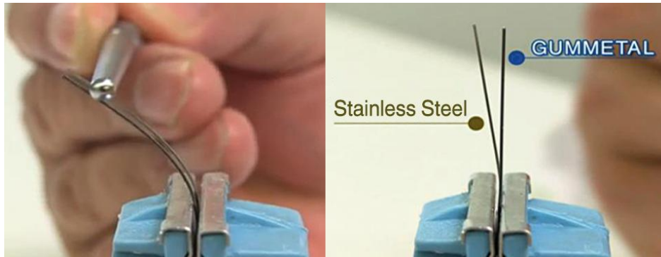
Fig. 1.32 The superior recoverable strain of Gum Metal wire compared to the one of conventional stainless steel wire after bending
