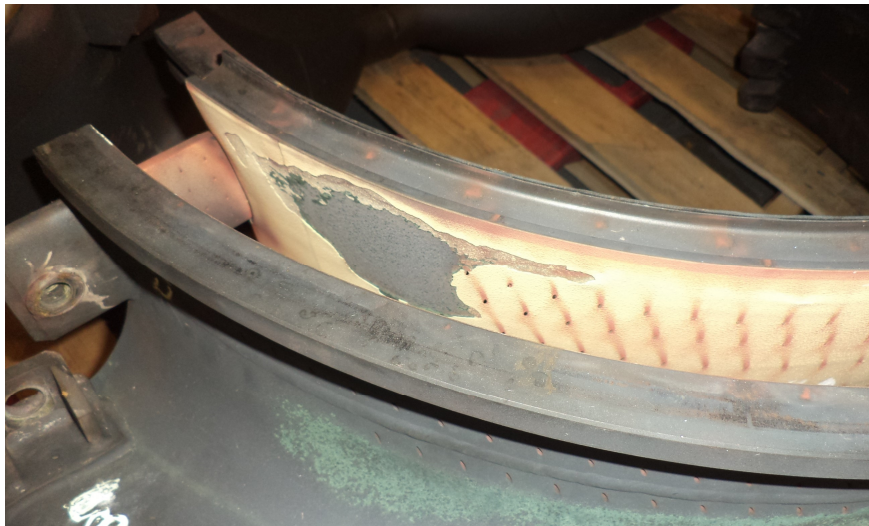
Fig. 45 Thermal barrier coating spallation found on the internal surface of the analyzed object after service.
