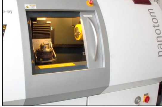
Fig.3.13 GE Phoenix Nanotom M tomograph used for micro-XCT scanning (MCL Leoben).
