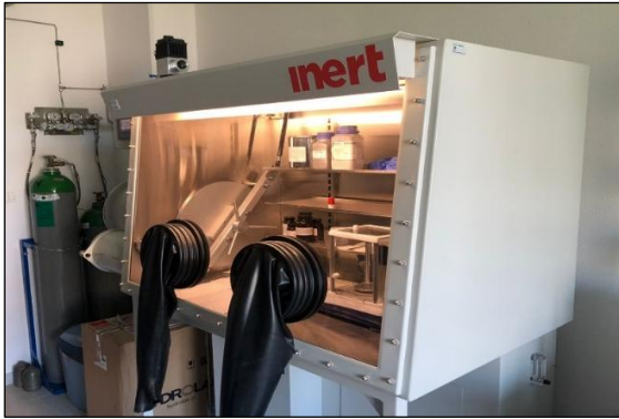
Fig.3.5 Glove box used for preparation of the starting powders (IPPT PAN).
