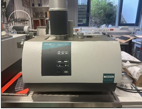
Fig.3.15 Thermal diffusivity measurement using Netzsch LFA 457 (Fraunhofer-IFAM Dresden).
