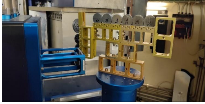
Fig.3.19 Mounting of samples for the measurement of residual stresses using neutron diffraction (ND) at Paul Scherrer Institute (PSI), Villigen. Switzerland.
