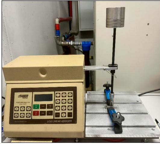
Fig.3.21 Taber Linear Abraser – Model 5750 (IPPT PAN).
