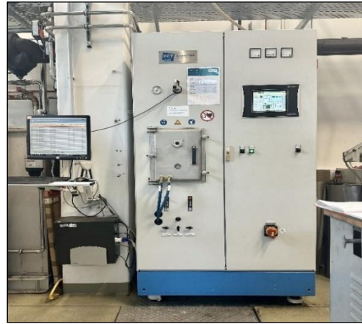
(a) Thermal Technology LLC hot press (IPPT PAN). (b) FCT Systeme GmbH device for spark plasma sintering (Fraunhofer-IFAM, Dresden).
