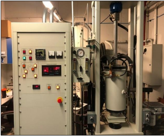
(a) Thermal Technology LLC hot press (IPPT PAN). (b) FCT Systeme GmbH device for spark plasma sintering (Fraunhofer-IFAM, Dresden).
