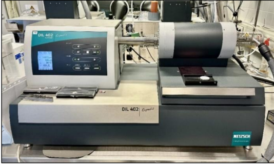
Fig.3.17 Netzsch DIL 402 Expedis classic dilatometer used for the measurement of CTE at Fraunhofer-IFAM Dresden.
