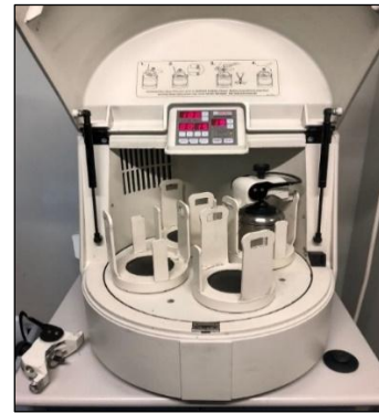
Fig.3.6 Pulverisette 5 Fritsch planetary ball mill used to obtain powder mixtures (IPPT PAN).
