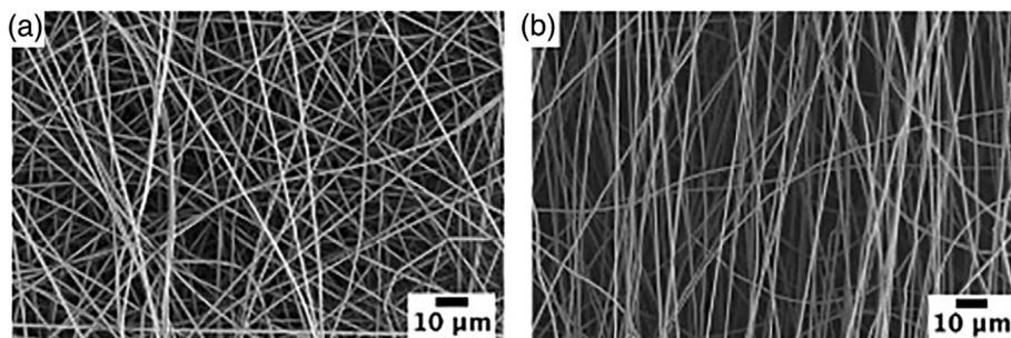
FIGURE 5 Scanning electron microscope (SEM) micrographs of (a) random, and (b) aligned poly(vinyl butyral-co-vinyl alcohol-co-vinyl acetate) (PVB) fibers
