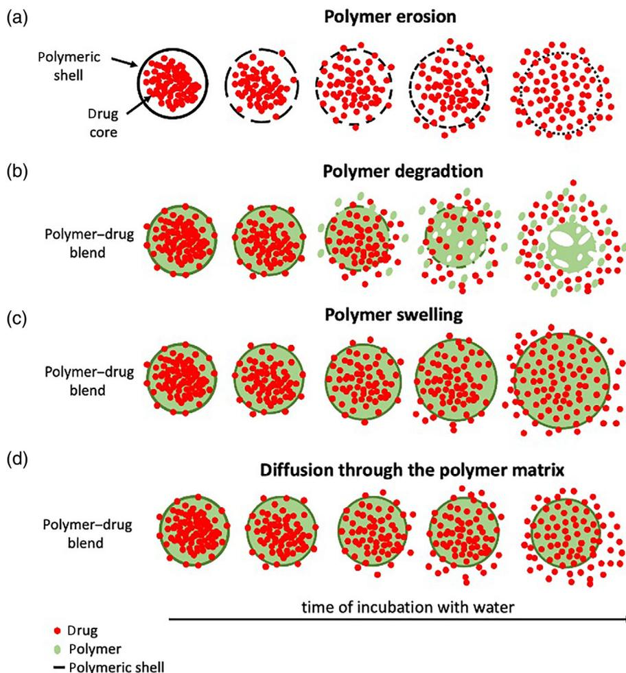
**FIGURE 8** Drug release mechanism from electrospun fibers through a polymer (the cross section of fibers): (a) erosion, (b) degradation, (c) swelling, and (d) diffusion through the polymer matrix
