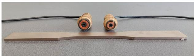
**Fig. 2** Sensor C18 (left), and C14 (right) on sample made of alumide-coated MAR-M247
