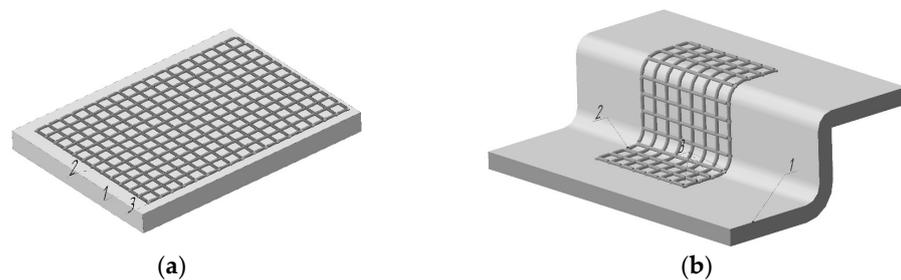
**Figure 11.** Surface schemes for restoring worn surfaces: (a)—flat, (b)—curved: 1—substrate, 2—reinforcing mesh, 3—intermediate adhesive layer (glue) [78].
