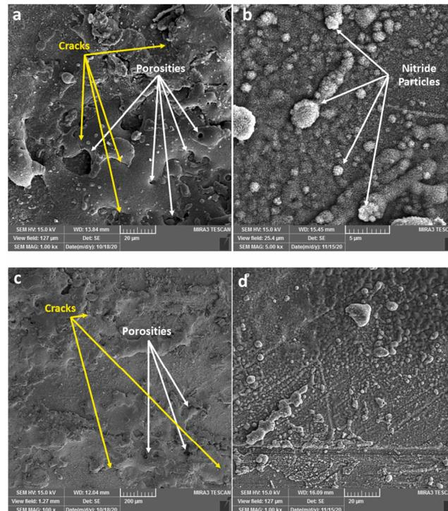
**Figure 15.** The morphology of the samples after ESA (a,c) and after ESA and modification by plasma nitriding (b,d), resulting in a smoother morphology and closing of the surface crack network. Substrate: 1045 carbon steel; alloying electrode: high-entropy alloy (HEA) AlCoCrFeMnNi; plasma nitriding parameters: 500 °C for 8 h, constant voltage of  $-600$  V [92].
