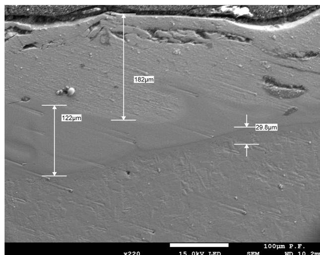
**Figure 12.** Microstructure of the coating (substrate–AISI 321) steel after sequential ESA T15K6 (discharge energy  $W_p = 0.55$  J), ESA T15K6 ( $W_p = 0.90$  J), and MPM deposition. MPM is a mixture of VK6 powder and a two-component epoxy system filled with Loctite 3478 ferrosilicon [80].
