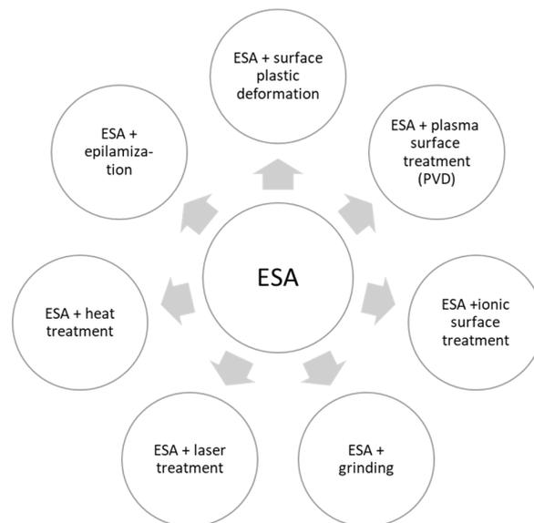
**Figure 4.** Directions for the development of combined (hybrid) technologies based on the ESA method.
