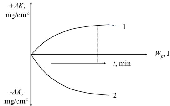
**Figure 2.** Change in weight of cathode (1) and anode (2) as a function of applied energy and treatment time.  $\Delta A$ —erosion of the anode;  $\Delta K$ —gain of the cathode;  $W_p$ —applied value of the energy of the spark discharges when depositing a substrate with an area of 1 cm<sup>2</sup>.
