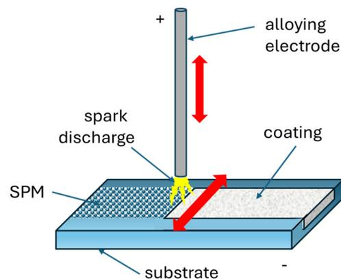
**Figure 3.** Scheme of the electrospark alloying technology using a special process medium.
