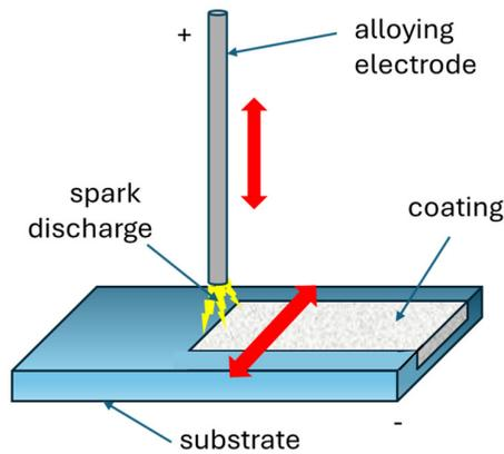
**Figure 1.** Schematic of the traditional electrospark alloying technology.
