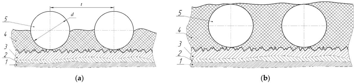
**Figure 10.** Restoration of worn surfaces of rotating bodies by the combined technology of ESA + MPM (wire reinforcement): (a) a schematic illustration of the stage of dipping the reinforcing wire into the MPM layer applied after ESA; (b) a schematic illustration of the completed coating, including the MPM layer reinforced with a wire layer. 1—part, 2—forming transition layer, 3—ESA coating made of hard wear-resistant metal, 4—metal-polymer material, 5—reinforcing wire [75].
