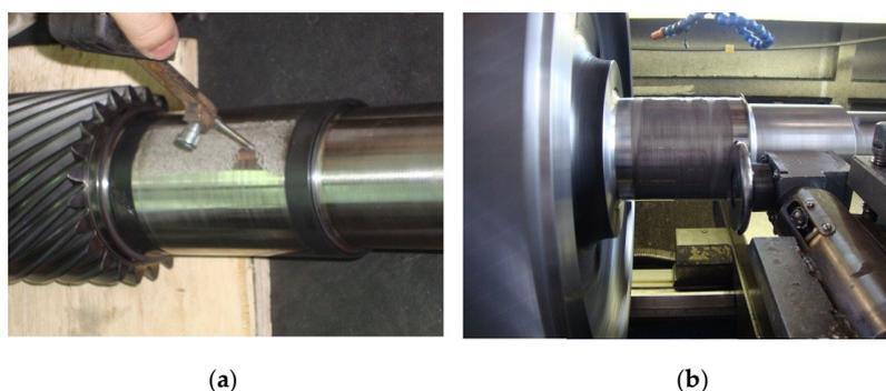
**Figure 18.** The ESA of the bearing journals of the gear shaft (a) and the SPD of the bearing journal of the gear wheel (b). The turbocompressor is a GTT-3 model manufactured by TRIZ LTD [97].
