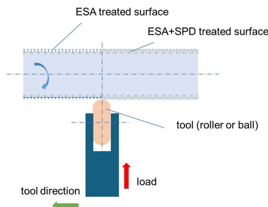
**Figure 5.** Scheme of the running-in process for ESA coatings.
