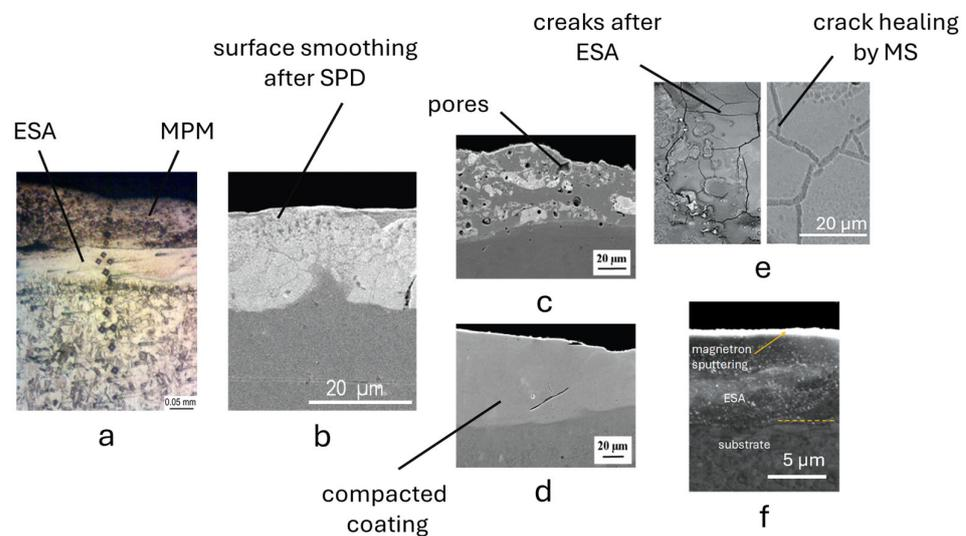
**Figure 16.** The effect of hybrid ESA technologies on coating morphology and microstructure: (a) ESA + metal-polymer material coating with imprints after microhardness testing; (b) ESA + surface plastic deformation coating; (c) ESA coating before laser treatment; (d) ESA + laser treatment coating; (e) surface of ESA + magnetron sputtering coating; (f) cross-section of ESA + magnetron sputtering coating.
