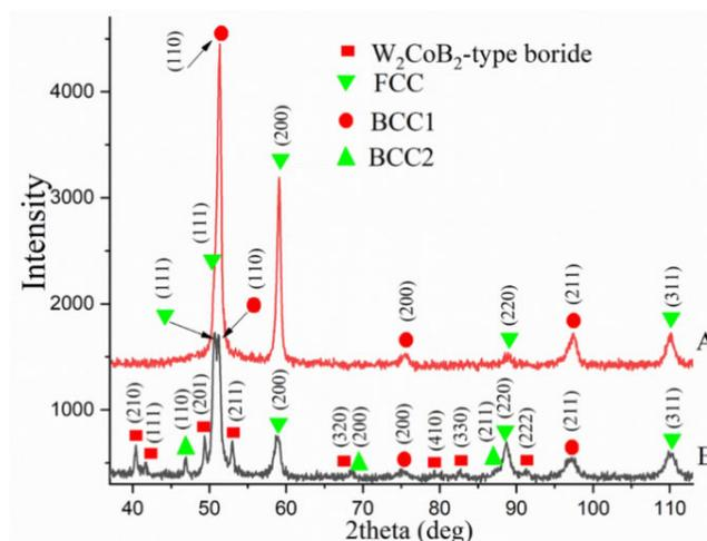
**Figure 8.** X-ray diffraction patterns of the as-cast alloys  $\text{Ti}_{0.5}\text{W}_{0.25}\text{Cr}_{0.5}\text{FeCo}_{1.75}\text{Ni}_3\text{Al}$  (A) and  $\text{Ti}_{0.8}\text{W}_{0.25}\text{Cr}_{0.5}\text{FeCo}_{1.75}\text{Ni}_3\text{AlB}_{0.6}$  (B) [70]. The alloys were produced by arc melting using metals with a purity of >99.5 at.% and titanium diboride powder.
