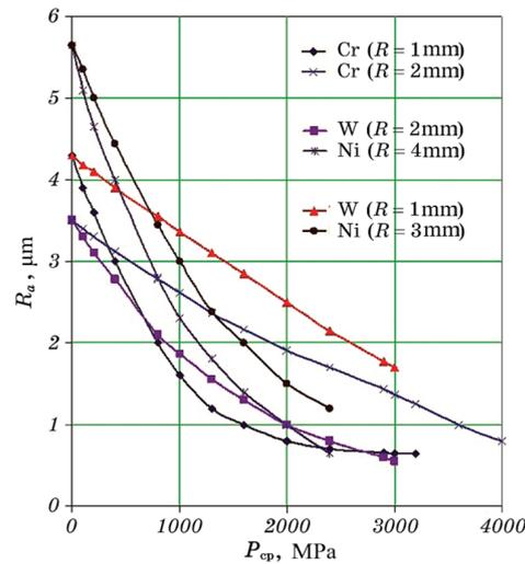
**Figure 6.** The surface roughness ( $R_a$ ) of steel 45 (carbon steel with a carbon content of 0.45%) after combined treatment (ESA with tungsten, chromium, and nickel, followed by DS) depends on the force ( $P_{cp}$ ) diamond smoothing (DS) at different radius of the diamond indenter ( $R$ ) [63].
