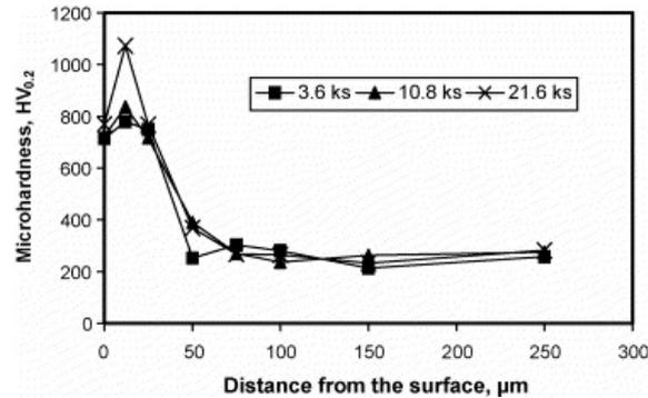
**Figure 14.** Influence of nitriding duration on the microhardness of cast iron samples coated by ESA (parameters of ESA: capacitor 150  $\mu$ F, voltage 50 V, alloying electrode: AISI-304 stainless steel [89]).
