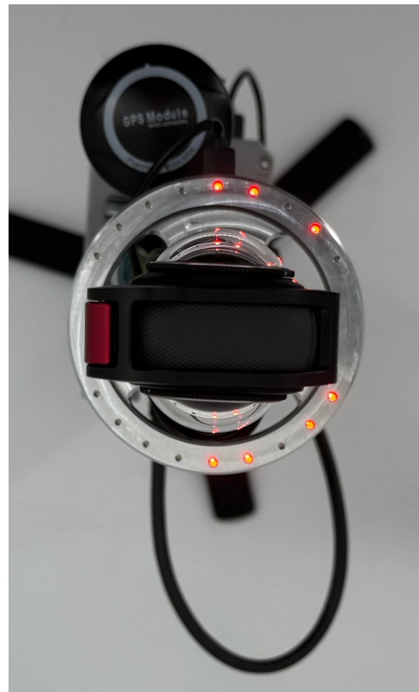
Figure 3: Affordable mobile mapping system - top view. Custom camera to LiDAR synchronisation based on leds showing timestamp with Gray code, an open-source can be found at https://github.com/MapsHD/MandeyeLedTimestamp .
