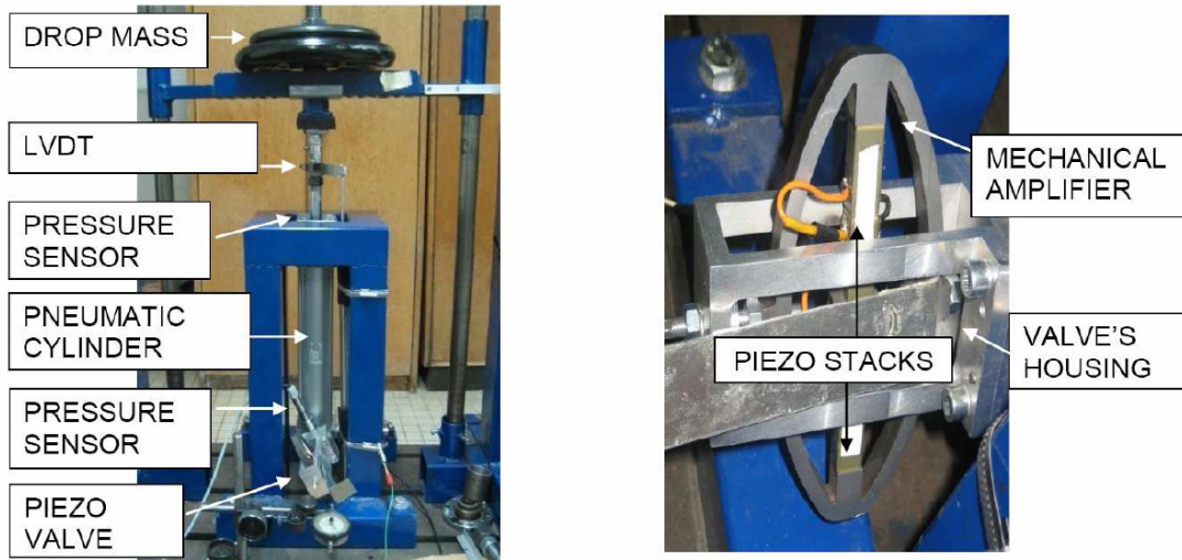
Figure 7 Experimental stand and piezo-valve.
