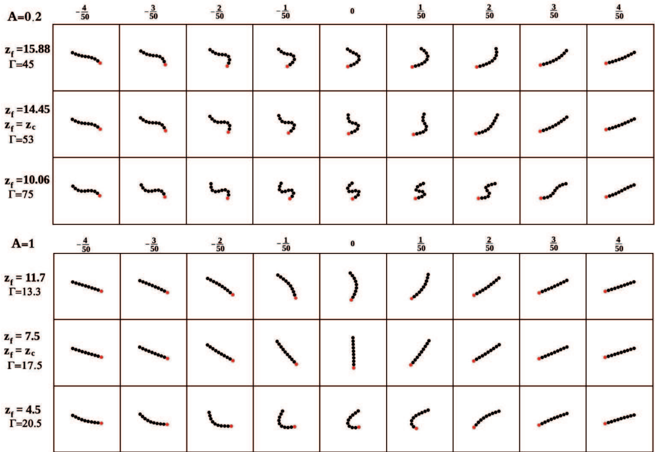
Fig. 14. Evolution of a fiber shape (drawn to scale) for N = 10 . Top: A = 0.2 . Bottom: A = 1 . Snapshots from simulations taken at the indicated times \bar{t}/\tau (with \bar{t} = t - t_f(2) and \tau = t_f(3) - t_f(2) , where t_f(n) is the instant of the n -th flip). The indicated values of z_f and \Gamma are attained at \bar{t} = 0 (second flip).
