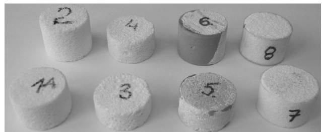
Fig. 5. Ceramic samples prepared for measurements in the impedance tube with diameter 29 mm; the samples 5 and 6 are made up with plaster, whereas the samples 7 and 8 are wrapped up in a thin tape in order to fit well in the tube.
