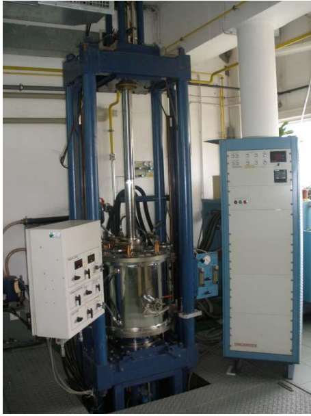
Fig. 1. Thermal Technology Astro uniaxial hot press
