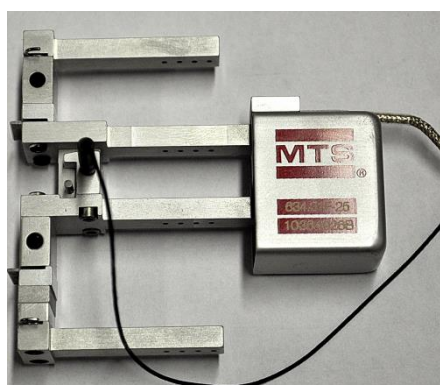
Fig. 3. Extensometer for measuring displacement
