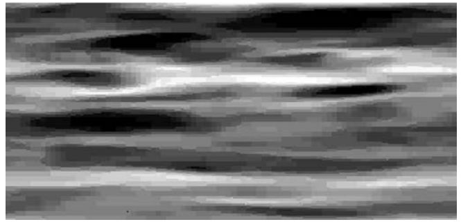
Fig. 6. Synthetic image of the wall temperature field generated from the DNS solution for water ( Pr=5.4 )
