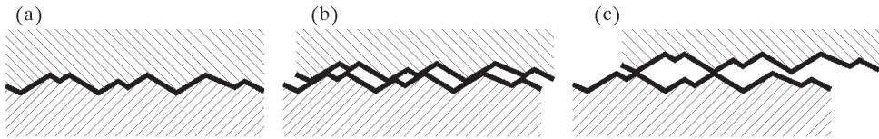
Fig. 14. Configurational dilation resulting from interaction of initially matching primary asperities: (a) u_t^s = 0, u_n^s = 0 ; (b) 0 < |u_t^s| < u_A, 0 < u_n^s < \delta_A ; (c) |u_t^s| > u_A, u_n^s = \delta_A
