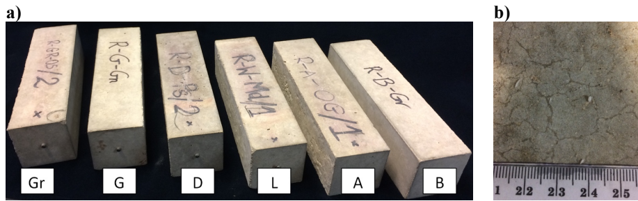
Fig. 2. Specimens subjected to 10 cycles of WD conditions, 10% of NaCl and 60°C: a) general view - one beam from each concrete, prismatic specimens 75x75x285 mm, b) surface view - with granite aggregate (G).
