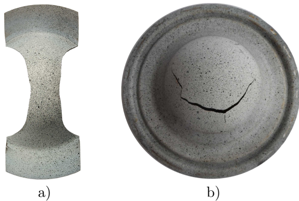
Figure 1. Sample fractured specimens: (a) 30 mm wide, (b) circular (180 mm diameter).
