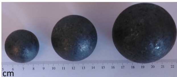
Fig. 4 Balls used for the tests: with diameters of 30 mm, 40 mm, and 50 mm
