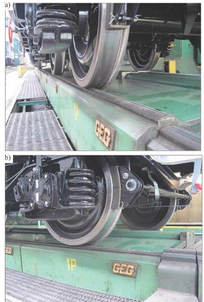
Fig. 2. Positions of suspension beams of measurement modules while conducting tests of freight wagon wheel forces – freight wagon twisting, (a) lifting the wheel over the zero level of the rail head (b) lowering the wheel in relation to the zero level of the rail head
