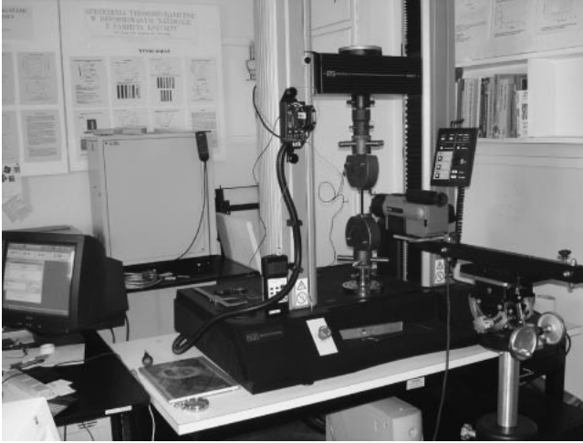
Fig. 2 Photograph of the testing equipment—with a specimen in testing machine and infrared camera.
