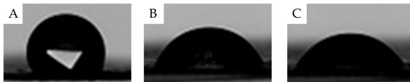
Figure 4. Contact angle images of the samples: (A) PU, (B) PU-NL, and (C) PU-NL/EEP.
