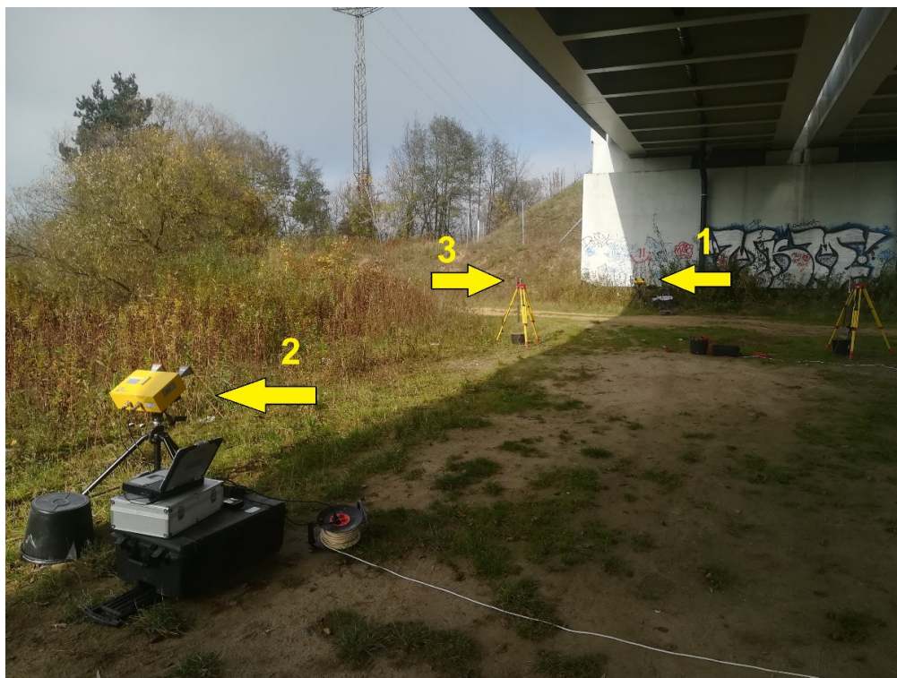
Figure 11. Bridge No. 2; 1—radar No. 1, 2—radar No. 2, 3—inductive transducer for the reference measurement.
