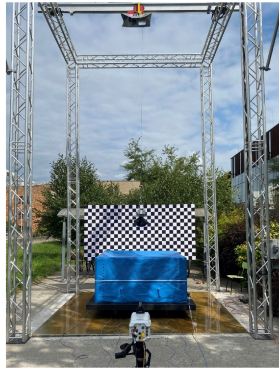
Fig. 1. The numerical model of a rescue air cushion, demonstrator in 1:2 scale and a dedicated drop stand during experimental tests.
