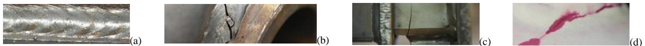
Fig. 2. Welding joints at inspection after fatigue tests: (a) splashes ( 2 \times 10^6 ), (b) crack in HAZ, weld and PM ( 1.5 \times 10^6 ), (c) crack in HAZ and PM ( 1.7 \times 10^6 ), (d) crack in weld and PM ( 2 \times 10^6 ), (HAZ – Heat Affected Zone, PM-parent material)
