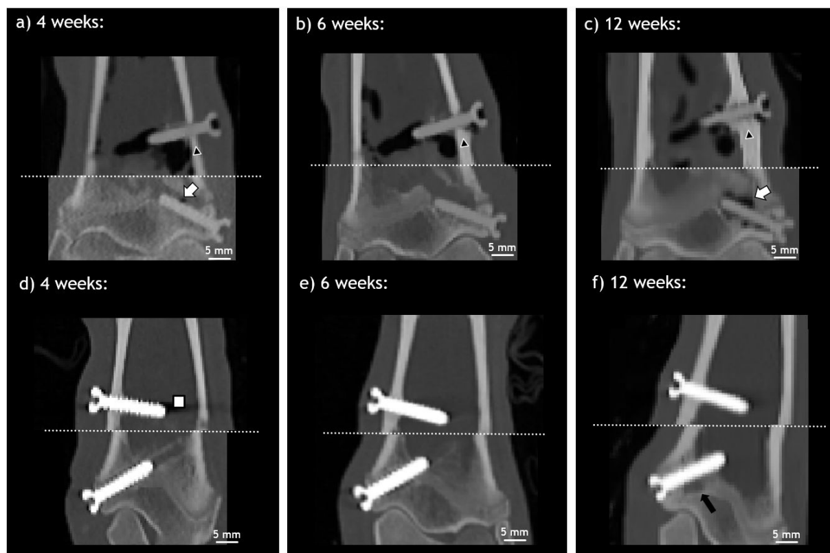
Figure 3: In vivo cCT images of distal tibiae of one animal. ZX00 (a-c) and Ti (d-f) screws 4, 6 and 12 weeks after implantation are shown. White arrows indicate gas formation around the epiphyseal screw (a, c). Cortical thickness increases over time (a-c; black triangle). Some scanning artefacts (white square) were detected around the Ti-screws, mainly at the screw tip 4 weeks after implantation (d). Slight change in trabecular bone structure was detected below Ti-screw after 12 weeks (f; black arrow).
