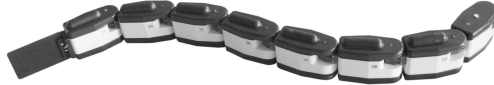
FIG. 1. A photograph of the modular AmphiBot robot constructed in the School of Computer and Communication Sciences, EPFL Switzerland ( https://www.epfl.ch/labs/biorob/ ).
