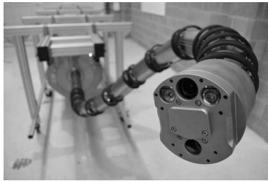
FIG. 2. Oliver Crispin Robotics Ltd.: a modular bionic trunk-like manipulator: an unsleeved, integrated X125 system with an inspection camera and light tool ( http://www.ocrobotics.com ).
