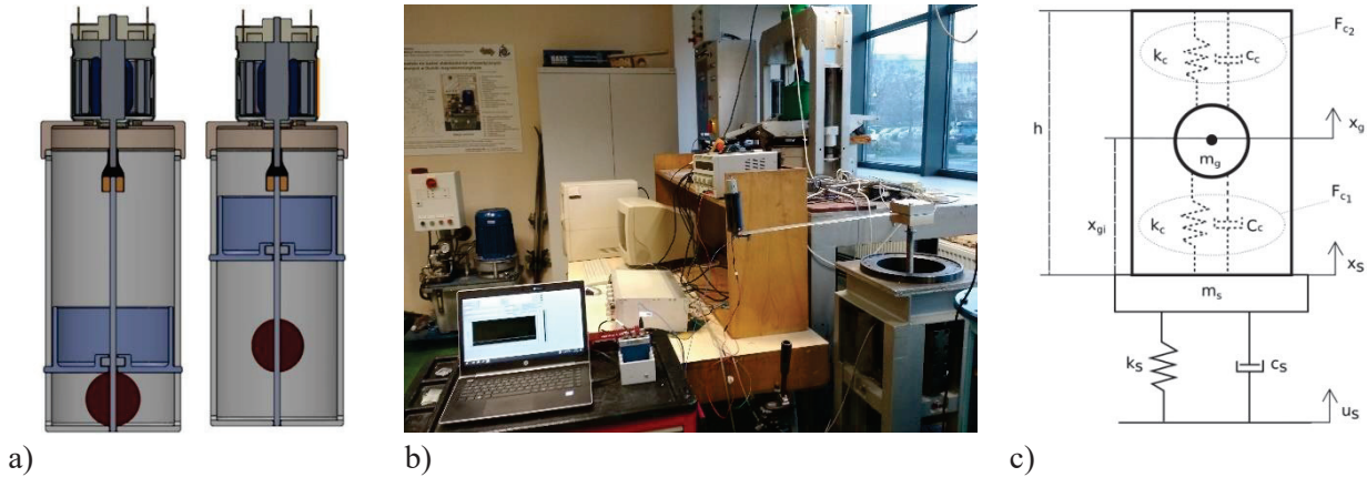
Fig. 1 a) ATPID model, b) Experimental test stand, c) Scheme of the ATPID construction
