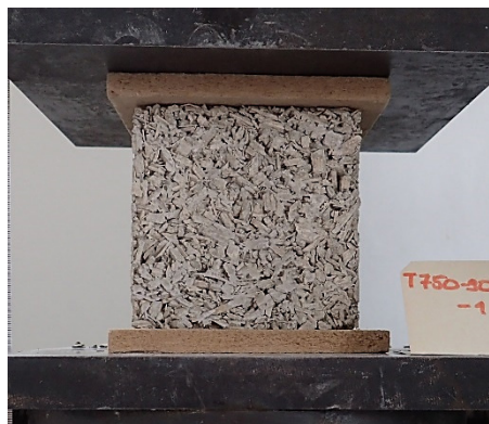
Figure 1. Compressive strength test of T750 hemp-lime composite
