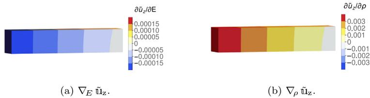
**Fig. 5.** Beam benchmark example. Sensitivity fields of the inverse elasticity problem (for the case provided in row 1 in Table 1).
