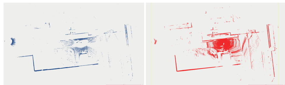
Figure 10. Undistorted, aggregated point clouds were built using data from the Livox Mid–40 with the rotated reflector (blue) and Velodyne VLP 16 (red) at Zwentendorf NPP. Top down view of Figure 9.
