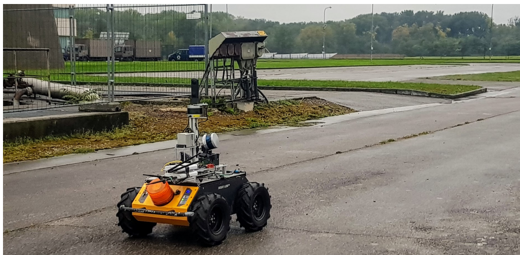
Figure 8. Robotic platform equipped with multiple mapping systems. This robot was used for the evaluation of the proposed contribution. The robot provided two 3D data streams for further comparison.
