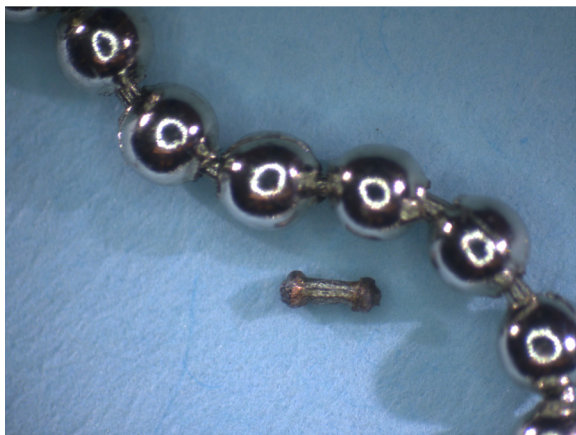
Fig. 2 A ball chain used in the experiments and a metallic dumbbell connecting consecutive metallic beads of the chain.
