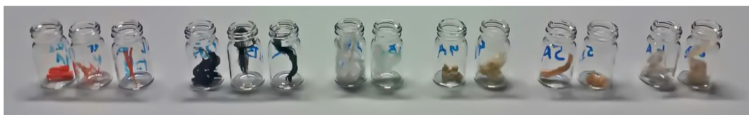
Fig. 2: The macroscopic view of six different pristine ropes and their samples weathered in the laboratory, on the right the same material new and after weathering with changes in colour and shape.
