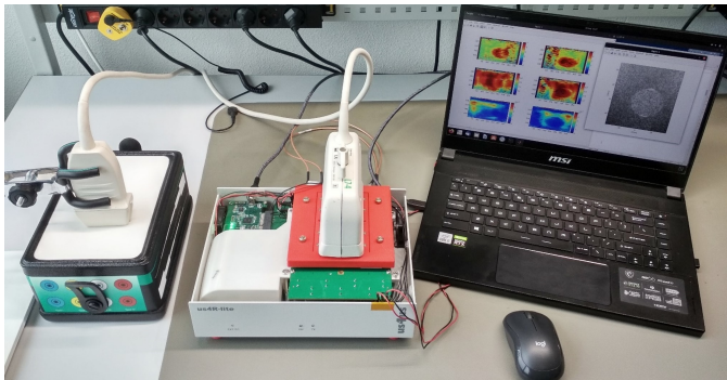
Fig. 1. The setup that was used in this work. Left to right: the ATL L7-4 probe over the CIRS 049A elastography phantom, the transmit-enhanced us4R-lite portable research platform connected to PC. Detailed description in the text.
