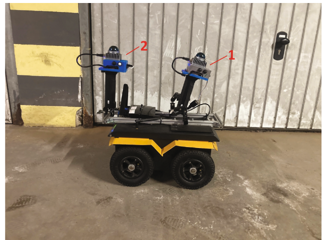
Fig. 7. System setup for accuracy, precision, robustness and repeatability assessment. 1: main LiDAR (3D map building and navigation), 2: physically mounted hand held mobile mapping system [20] for trajectory tracking and 3D map to ground truth data registration.
