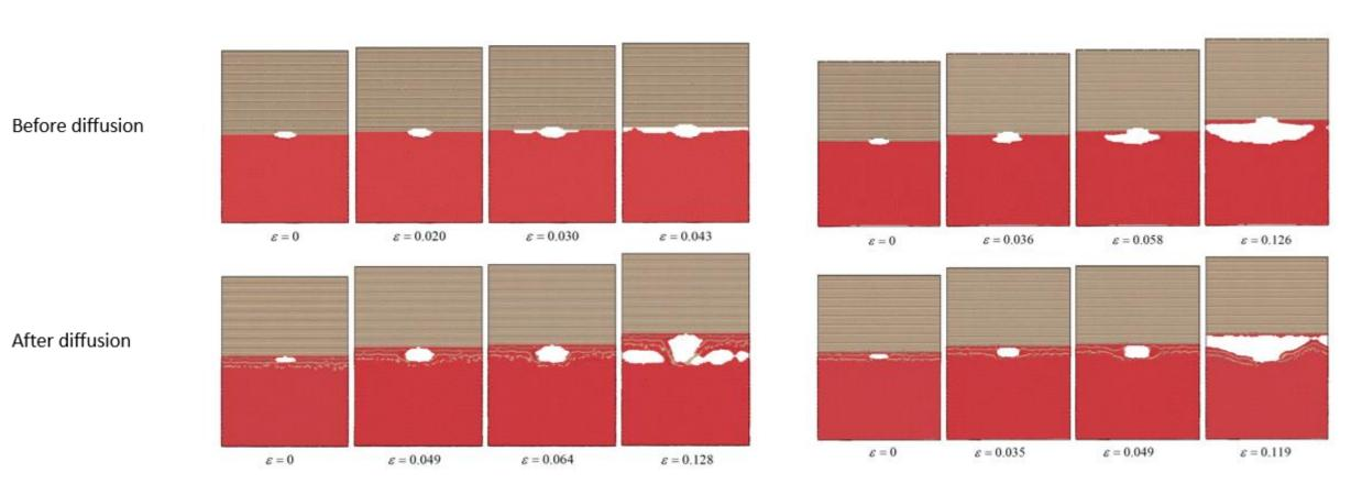
Si-terminated 6H-SiC/Al under pure tensile loading (mode I).
