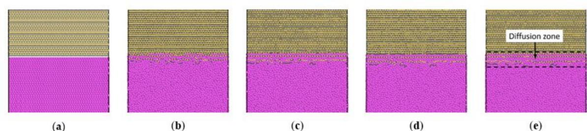
(b) (a) Cross-sectional views of the atomic configurations of C-terminated 6H-SiC/Al interface. (a) Atomic structure at 300 K before relaxation and the configuration after maintaining the system at 2000 K for (b) 0 ns, (c) 2 ns, (d) 4 ns and (e) 6 ns.
