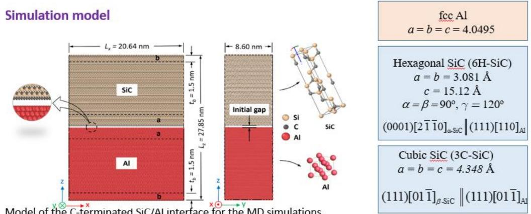
Model of the C-terminated SiC/Al interface for the MD simulations.
