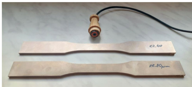
Fig. 2 Pot-core probe and specimens of MAR 247 nickel-based superalloy with 20 μm and 40 μm thick aluminide coatings
