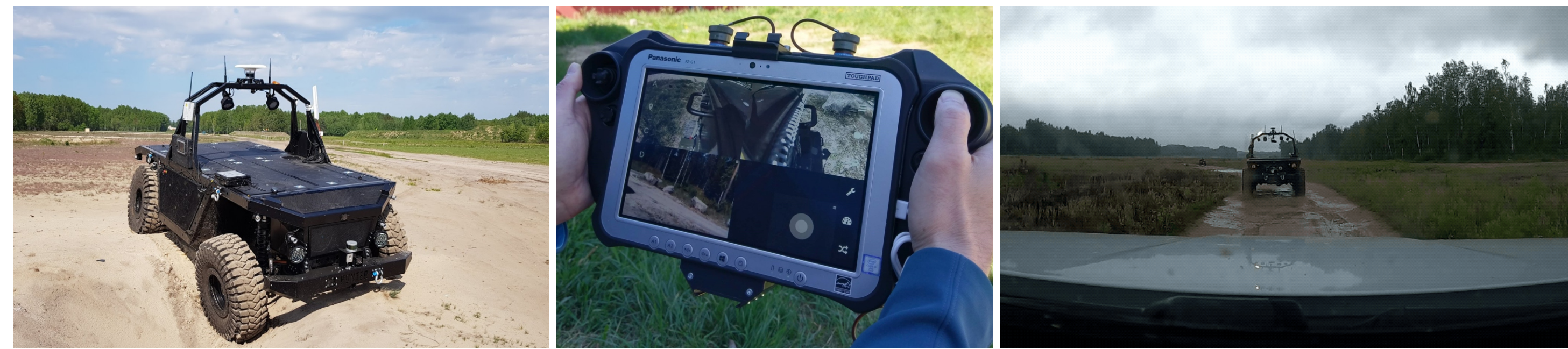
Modular autonomous system – original drive-by-wire system for FORD Ranger
