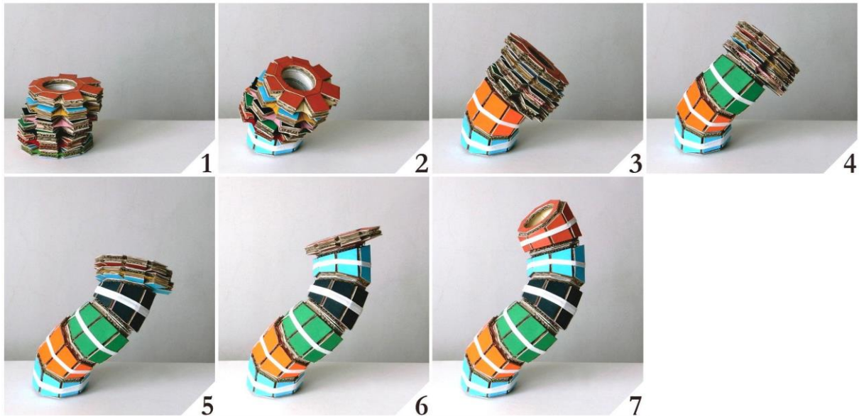
Fig. 4. A sequential deployment of a Pipe-Z spiral comprised of six octagonal foldable modules. The deployed units gain quasi-rigidity from the white compression bands.
