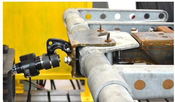
Fig. 1. A mechanical connection of the servo-motor and towing frame (for the recovery vehicles to highways and expressways), through a spherical grip and A50-X coupling ball.
