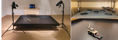
Fig. 2. Experimental stand: plate, ferromagnetic magnets applied for magnetic anomaly generation and mobile platform with IMU and magnetometer.
