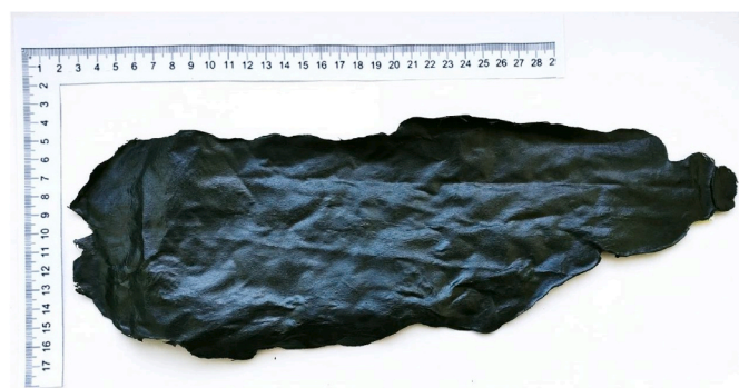
Fig. 1. Image of GO paper fabricated in this study. (A colour version of this figure can be viewed online.)
