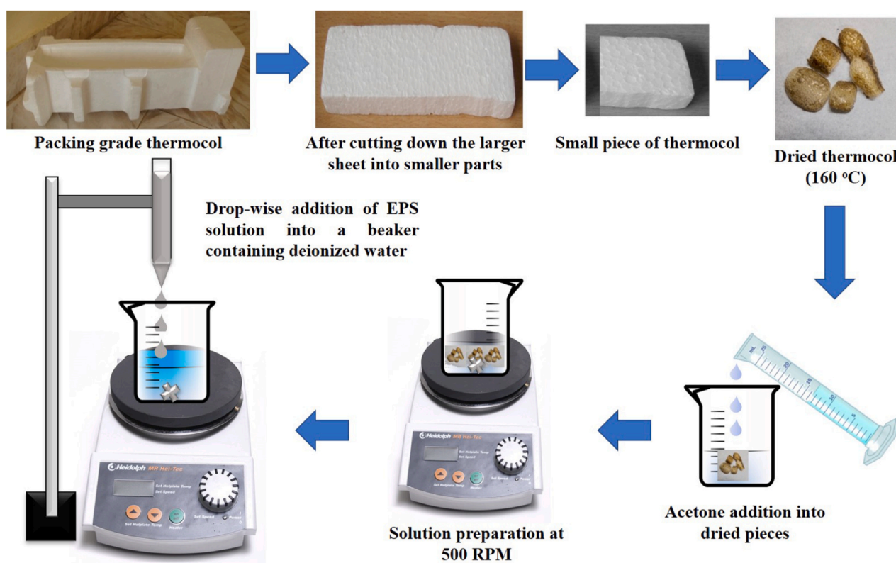
Fig. 1 – Schematic representation depicting the process of nanoparticle synthesis using EPS waste.
