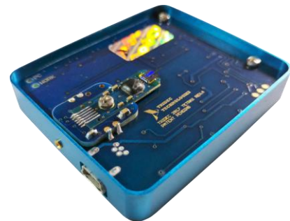
Fig. 2. Photograph of the lateral force calibration device for TetraX atomic force microscopes, in which we use fabricated sensors
