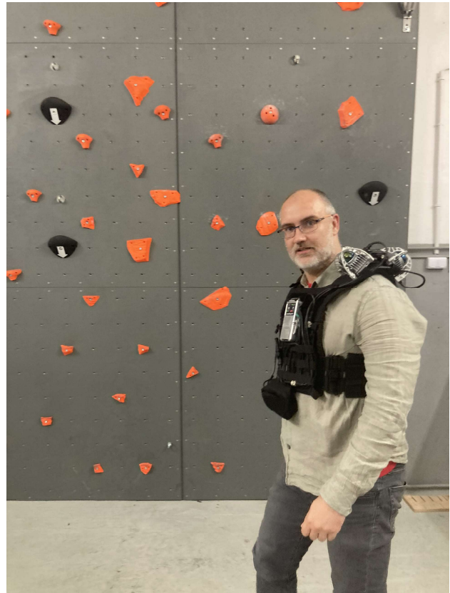
Figure 2. Configuration 1: Mobile mapping system mounted on the shoulder.
