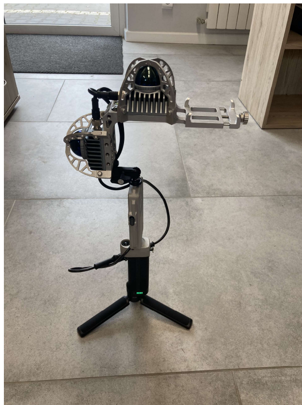
Figure 4. Configuration 4: Hand held mobile mapping system.
