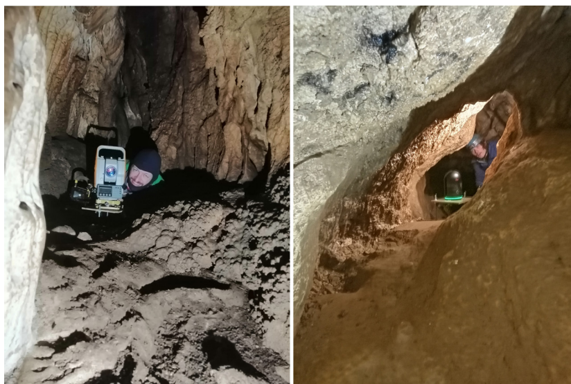
Fig. 4. Survey conducted in 2022. on the left - using a total station, and on the right - using a static laser scanner (Leica BLK 360).
