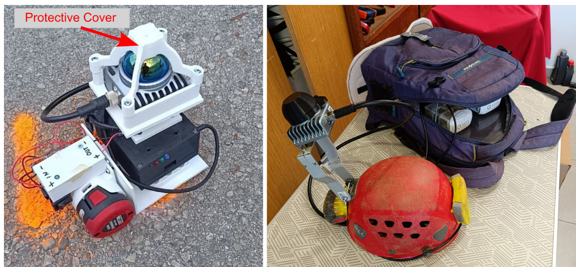
Fig. 2. Mandeye LiDAR system for mobile cave mapping: the handheld version for confined spaces (left) and the helmet-mounted version for hands-free operation in larger cave sections (right).
